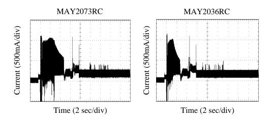
Figure 4.7 Current waveform (+12V DC)
