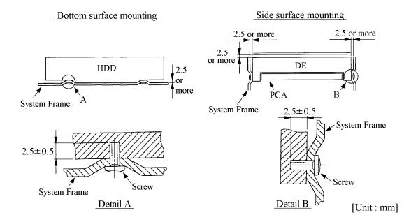
Figure 4.3 Mounting frame structure example
