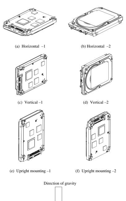
Figure 4.2 HDD orientations
