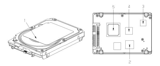
Figure 4.5 Surface temperature measurement points
