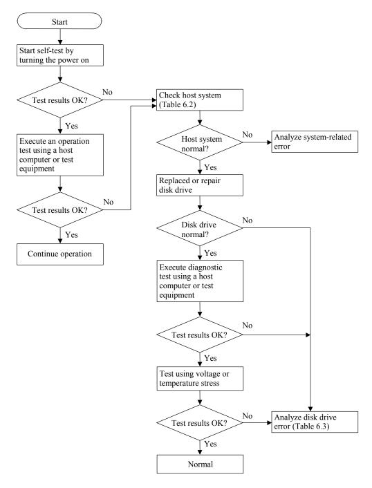
Figure 6.3 Test flowchart
