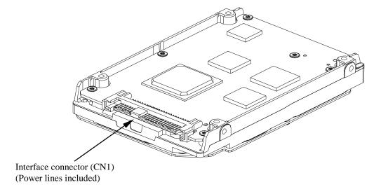
Figure 4.9 Connector location
