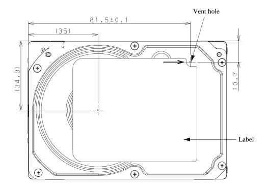
Figure 4.4 Vent hole location
