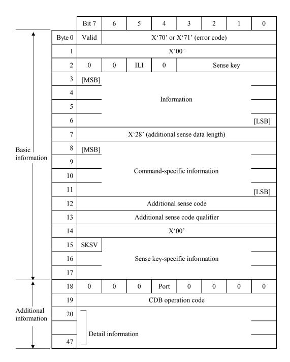
ILI: Incorrect Length IndicatorMSB: Most Significant ByteLSB: Least Significant ByteSKSV: Sense Key Specific Valid
