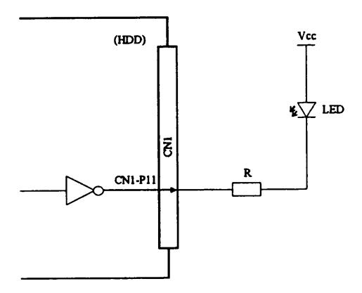
Figure 4.11 Recommended external circuit for Ready LED output
