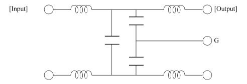
Figure 4.8 AC noise filter (recommended)
